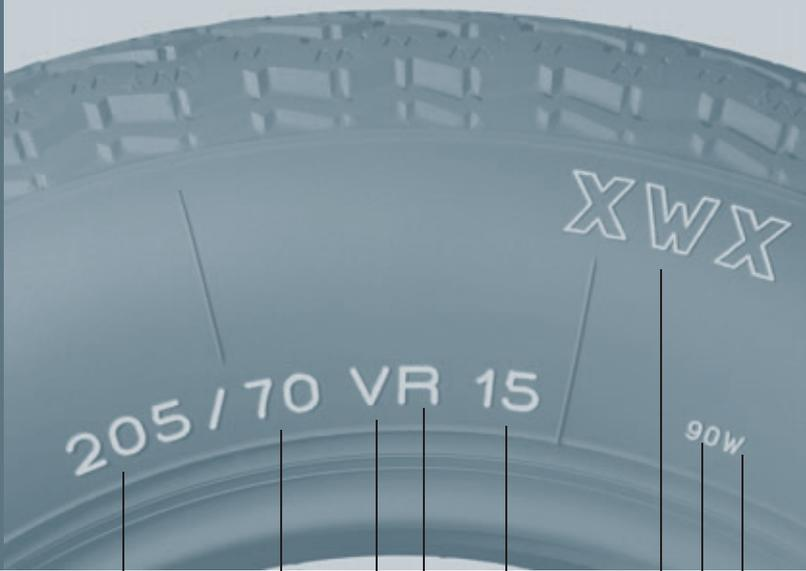
tyre width in mm      Aspect ratio      "R" for Radial      Nominal rim diameter in inches      Tread pattern      Speed index VR > 210 km/h      Speed index 270 km/h
